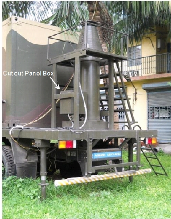
Fig. 2a : Instrumentation Cabin on the vehicle with mast
