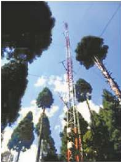
Fig 2: 50 (Left) m tall tower (Flux-tower) equipped with Eddy-Covariance system for continuous monitoring of Greenhouse Gas flux at high altitude Himalayan conifer forest at Dhotrey forest, Darjeeling; (Right) CO 2 exchange between biosphere and atmosphere and soil
