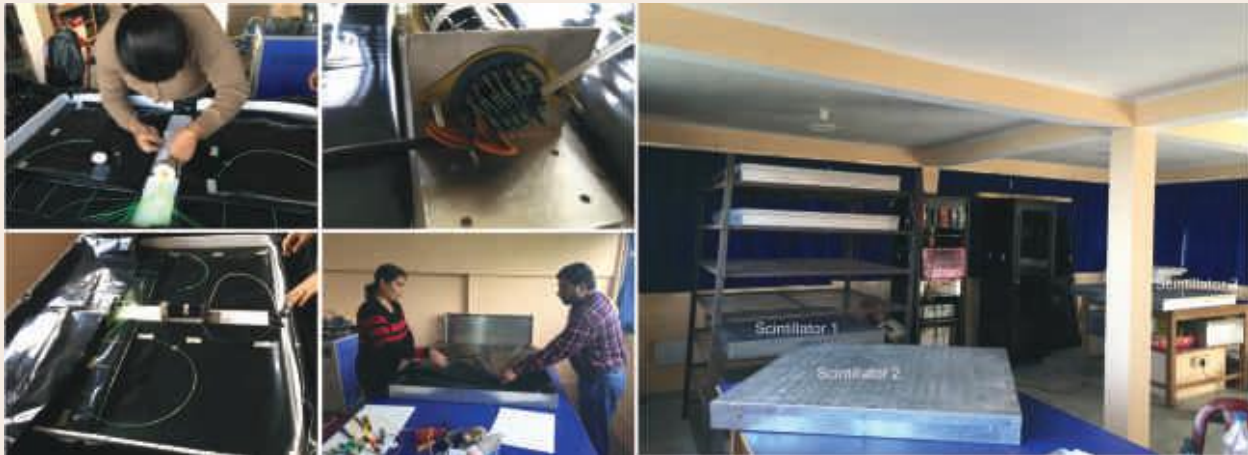
(Left) Steps of scintillator detector fabrication. (Right) Horizontal stack of three scintillator detectors to measure cosmic ray shower.
