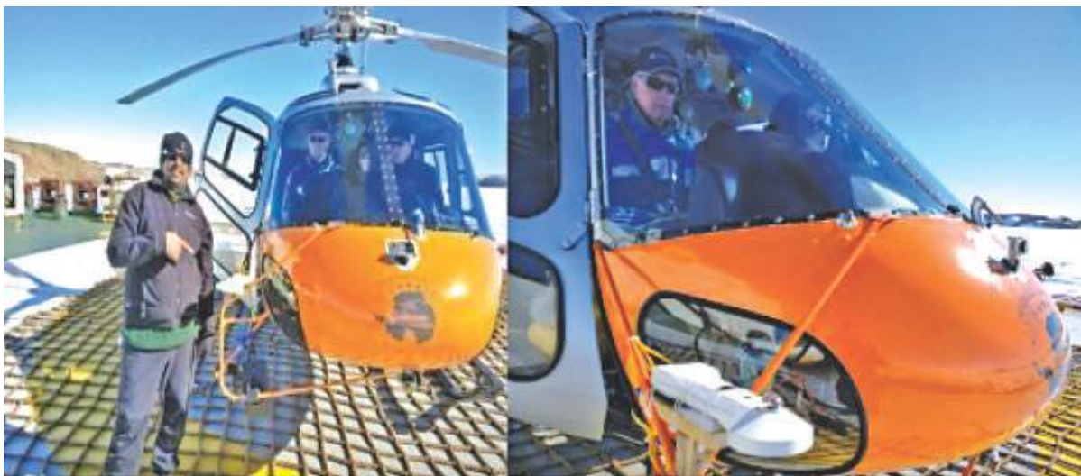
LHS figure shows the observer from Bose Institute, Dr. Sanat Kumar Das indicating first time the novel and unique set up of the experiment using a helicopter for in-situ measurement of intensities of solar radiation at different altitudes over Eastern Antarctica. RHS figure shows the image zooming over the Pyranometer installed in front of the helicopter .
