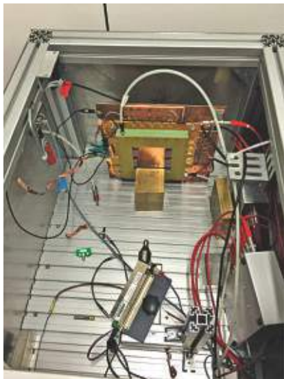
(Left) The experimental set-up with the X-ray generator (at GSI). (Right) Anode current per unit area as a function of X-ray generator voltage.
