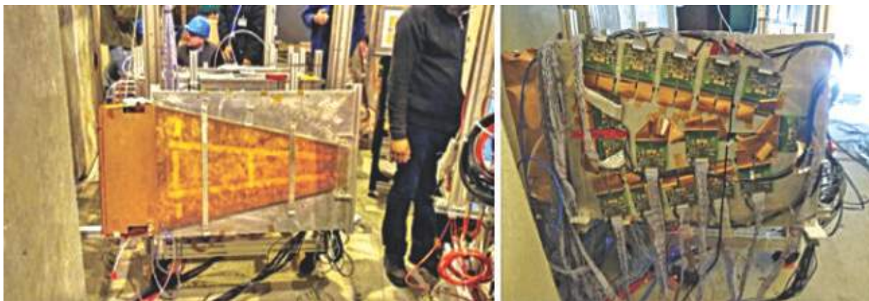
Figures above show a real size cooling plate (left), GEM chamber mounted on one side of the cooling plate (middle) and electronics mounted on other side of the cooling plate (right).
